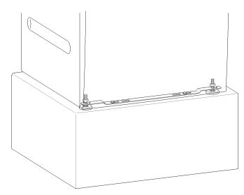
The anchors provided can be used to bolt the machine to the floor by both front feet. The fixing material provided is intended to be used for bolting the machine to a concrete floor.
