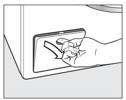
■ Open the drain pump access panel.
