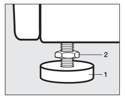
■ Using the open spanner supplied, turn counter nut 2 in a clockwise direction. Then turn counter nut 2 together with foot 1 to unscrew.
