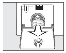
■ Remove the drain filter completely.
