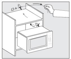
Slide the appliance into the housing unit. Feed the cable with the plug through the back of the furniture unit.
