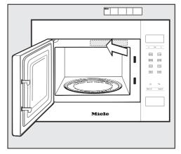
Stick the enclosed quick start guide to the frame behind the door as illustrated, making sure it does not block any of the vents. When building in the appliance, ensure that there is adequate ventilation to the front of the appliance.
