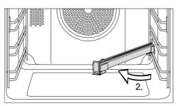
Then hold the FlexiClip runner at an angle towards the middle of the oven compartment (2.).
