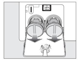
■ Remove the drain filters completely.
