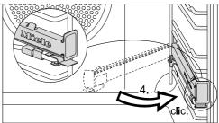
Then swing the FlexiClip telescopic runner back to the side and secure it to the top rail with an audible click (4.).
