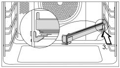
Slide the FlexiClip telescopic runner at an angle along the top rail as far as it will go (3.).
