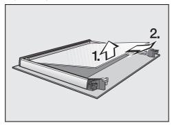
Then lift the bottom of the two middle panes up carefully and take it out.
