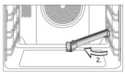
Then hold the FlexiClip telescopic runner at an angle in towards the middle of the oven compartment (2.).
