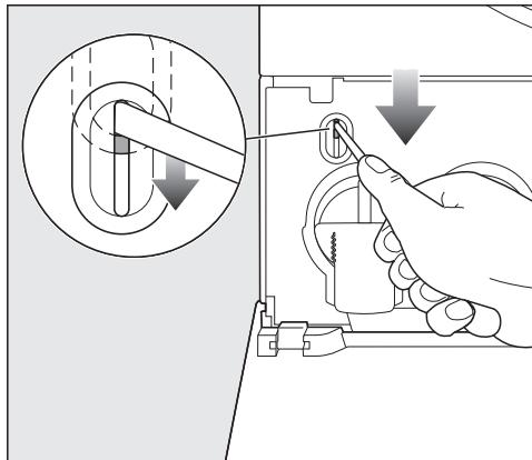
1. Use a screwdriver to push the door release mechanism all the way down without touching or opening the door.
