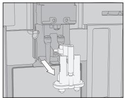
Grip the dispensing unit by the sides and pull it down to remove it.
