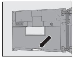
The drip tray is located at the bottom on the inside of the appliance door.
