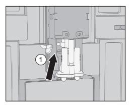
■ Detach the milk pipework from the dispensing unit as follows: pull the pull tab ① to the left.
