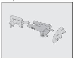
■ Take the dispensing unit apart, separating it into 3 components: the Y-piece, the spouts, and the holder.
