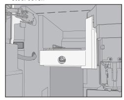
Remove the milk valve cover. Press on the recessed grip to unlock the cover. On the top right-hand side of the cover, you will find a pin for swiveling the cover out.
