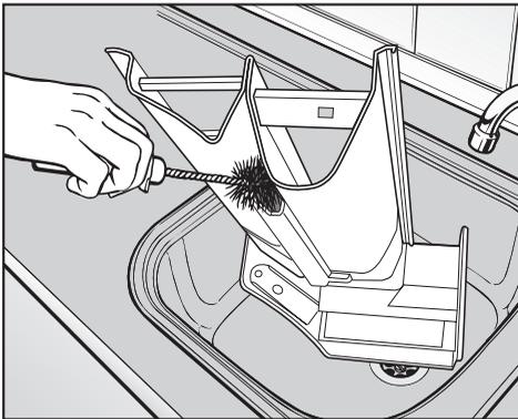
■ Clean the fabric conditioner channel using a brush and warm water.
