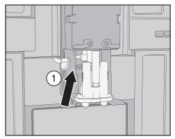
■ Detach the milk pipework from the dispensing unit as follows: pull the tab ① to the left.
