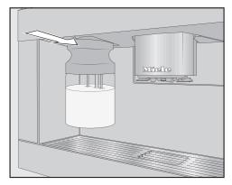
Push the milk container back into the coffee machine until it clicks into place.
