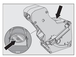
Wipe any coffee grounds from the filters. One filter is located in the funnel and the other to the left of the funnel.
