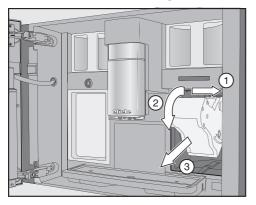
■ Pull the brew unit to the side ① first and then pull out to the front ③. Tilt the brew unit forward ② while doing so.
