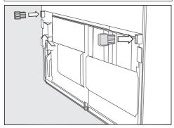
Fit the wall spacers onto the back of the refrigeration appliance on the bottom left and right.
