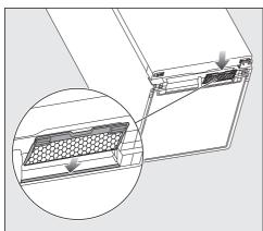
Place the rear edge of the insect protection grille in the rear channel of the opening.
