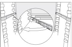
Attach the two adapters to the support ribs on the left and right at the desired height.
