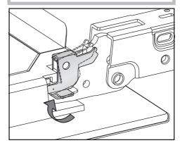
■ To relock the locking clamps, turn them back up to the horizontal position as far as they will go on both door hinges.
