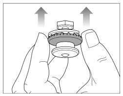
After cleaning the browning/broiling element, push the pressure cap back up using the outer ring of the pressure cap.
