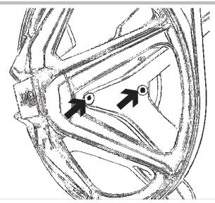
Use grease nipples to lubricate the drum shaft bearings with Arcanol L 100 grease after approx. 1,000 operating hours.
