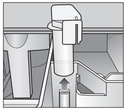
■ Remove the siphon. Clean the siphon with hot water and reinsert it.
