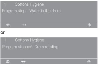
**Tip:** To open the door, press the "Water drain"  $\downarrow \downarrow j$  function button or select the "Extra Spin" program and press the "START" button.
