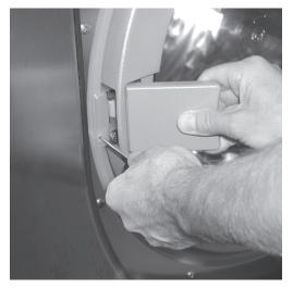
First insert the screwdriver into the opening next to the door lock, press it in, and hold it. Press against the door handle with your right hand and then pull the door handle to open the drum door. Never use force to open the drum door! Remove the laundry.
