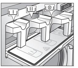
■ For standard wash programs, add powder detergent for the main wash to the Ш compartment and if desired, add detergent for a pre-wash to the ∐ compartment. Add fabric softener to the front of the 1<sup>(B)</sup> compartment.
