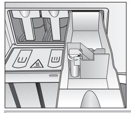
Do not fill the  $\underline{\mbox{\sc blue}}$  compartments above the level marker with liquid agents.
