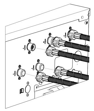
Before attaching the inlet hoses to the machine, the filters and seals included in the accessory pack must be inserted.
