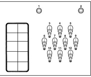
Connections **1** and **2** are provided for viscous agents. These connectors are sealed and need to be drilled open using an 8 mm drill bit.
