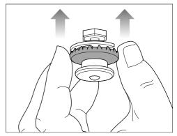
After cleaning, push the browning/grill element back up using the outer ring of the pressure cap.
