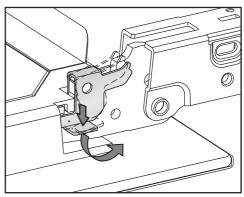
Release the locking clamps on the hinges by pushing them down as far as they will go until they are at an angle.
