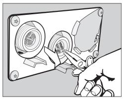
■ Use pointed pliers to grip the bar and pull out the filter; then clean the filter. Reassemble in reverse order.
