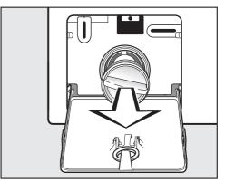
Remove the drain filter completely.
