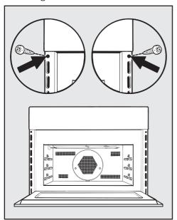
■ Open the door and use the screws supplied to secure the oven to the side walls of the housing unit through the holes in the oven trim.
