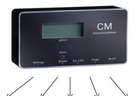
Rotary selector: Buzzer: Connection: Connection: Connection: switchpoint On/Off Ext. LED Sensor unit AC adapter
