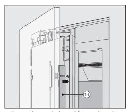
■ Press the angle bars ③ into the white plastic frame on both sides and screw them on loosely at first. Spare screws are provided in the plastic bag marked with the letter E.
