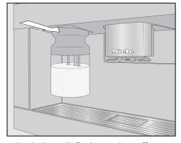
Push the milk flask into the coffee machine until it clicks into place.
