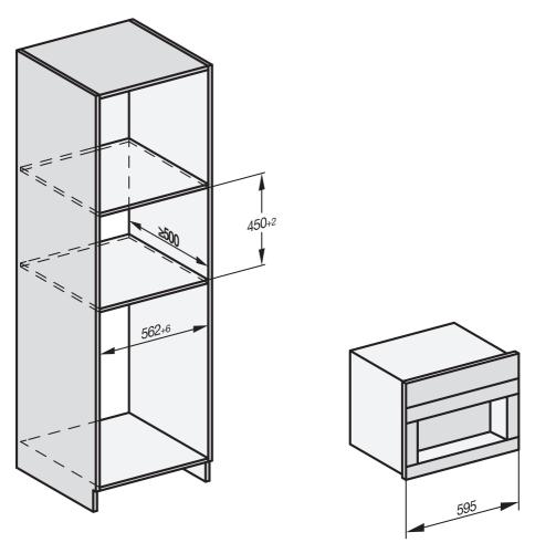
Combination with other Miele built-in appliances is possible. If the coffee machine is to be built in above another appliance, there must be a full-width, closed shelf between them. If the appliance is to be combined with a Gourmet warming drawer/built-in vacuum sealing drawer, no intermediate shelf is required in between.
