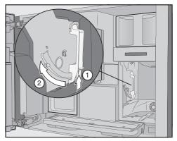
■ Press the button under the handle of the brew unit ① and, whilst doing so, turn the handle to the front ②.
