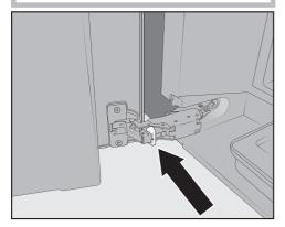
■ Remove the door opening limiters from the hinges by levering them out with a screwdriver, for example.
