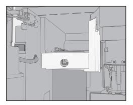
Remove the milk valve cover: press on the recessed grip to unlock the cover. On the top right-hand side of the cover there is a pin which enables you to swing open the cover.
