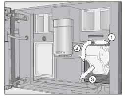
■ Pull the brew unit to the side ① first and then pull out to the front ③. Tilt the brew unit forwards ②.
