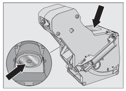
■ Wipe any remaining coffee residues from the filters. One filter is located in the funnel and the other to the left of the funnel.
