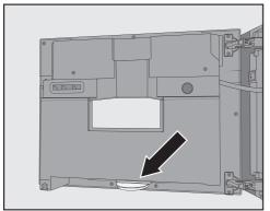
At the bottom of the inside of the appliance door there is a drip tray. Clean the drip tray regularly.
