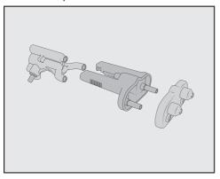
Dismantle the dispensing unit into 3 pieces: disconnect the Y-shaped piece, the dispensing spouts and the holder from one another.
