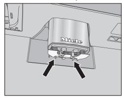
Push the two locking catches together (see arrows). The cup rim sensor will be released.
