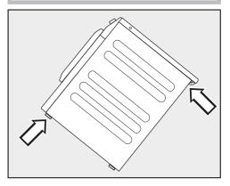
■ Carry the washing machine by the front feet and by the lid where it protrudes at the back of the appliance.
