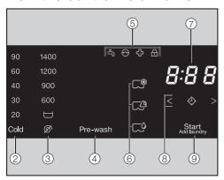
The ②, ③, ④, ⑥, ⑧ and ⑨ sensor controls react to fingertip contact. If a sensor control is illuminated, it can be selected.
