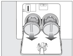
■ Remove the drain filters completely.
