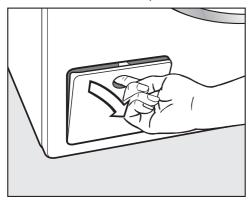
■ Open the drain pump access panel.
