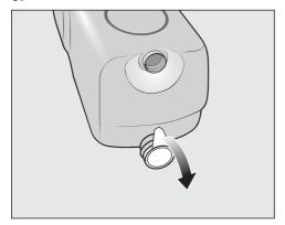
Remove the film seal from the cartridge completely.
