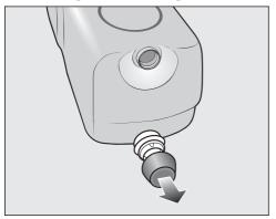
Remove the cover cap from the cartridge.
