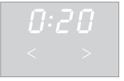
■ Touch the < or > sensor control repeatedly until the required programme running time appears in the time display.
