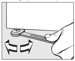
**Tip:** Use a spirit level to ensure correct alignment.
