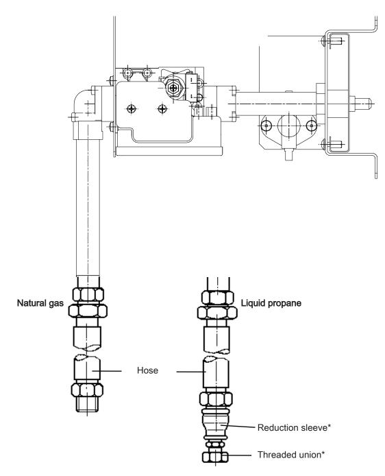
\* Supplied with the kit for converting natural gas to propane (LP).
