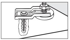
The material provided is intended for use in bolting the machine to a concrete floor. If other floor types are present at the installation site, the fastening material must be ordered separately.
