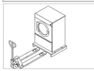
At the installation site, the tumble dryer must be lifted from the transport pallet using suitable lifting gear.
