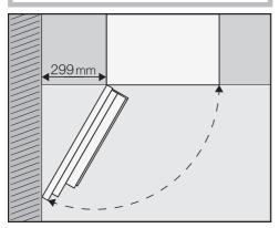
**Tip:** If a gap of at least 299 mm is maintained between the wall and the coffee machine, you will be able to open the appliance door wider, making the machine easier to use. For instance, it will be easier to remove the left-hand bean container.
