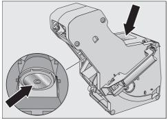
Wipe any coffee residue from the filters. One filter is located in the funnel and the other to the left of the funnel. The process of removing the brew unit causes ground coffee to drop onto the drip tray.
