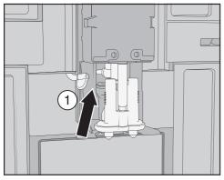
Detach the milk pipework from the dispensing unit as follows: pull the opening tag 1 to the left.
