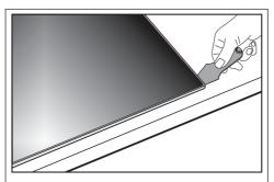
To remove the ceramic glass top, insert the scraper supplied in the corner between the frame and the worktop.
