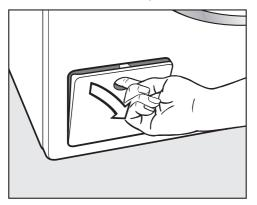
■ Open the drain pump access panel.
