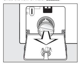
■ Remove the drain filter completely.
