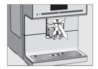
Carefully pull the stainless steel cover off and then pull the dispensing unit off towards you.
