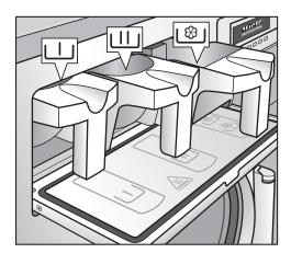
■ For standard wash programmes, add the detergent for the main wash to the Ш compartment and, if desired, add detergent for a pre-wash to the U compartment. Add fabric softener to the front of the 🐿 compartment.
