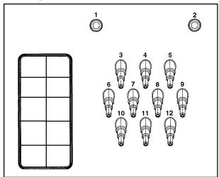
Connections 1 and 2 are provided for viscous agents. These connections are sealed and need to be drilled open using an 8 mm drill bit.
