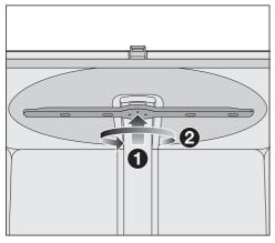
Push the upper spray arm upwards 1 to engage the inner ratchet. Then unscrew the spray arm by rotating the screw thread anti-clockwise 2 (view from below).
