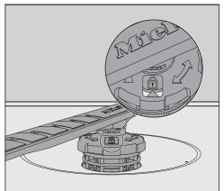
■ Rotate the screw thread clockwise until the arrow in the viewing window points to the lock symbol ⊕.
