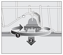
Rotate the screw thread of the middle spray arm clockwise 1 (view from above) and remove the spray arm 2.
