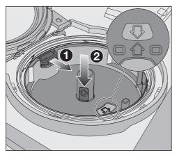
Pull the yellow pull tab in the direction of the arrow ① and reinsert the PowerDisk holder ② at the same time. To do this, the arrows in the PowerDisk holder and in the viewing window must point towards each other. The holder must lie flat. The AutoDos lid must close tightly so that the detergent powder does not get wet and clump together.
