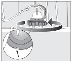
Replace the middle spray arm and turn the screw thread anti-clockwise (view from above) until it engages. Make sure that the recesses in the lock line up.
