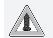
Screw the feet in before moving the dishwasher.
