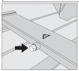
■ To measure the wash pressure, replace the blind stopper with a Luer Lock adapter.
