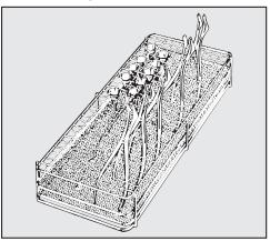
■ To ensure coverage of all surfaces by the wash liquor please open speculum and place in the insert.
