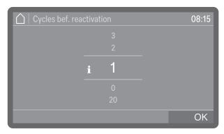
Cancelling machine lock due to lack of salt If the salt in the water softener has been used up, a fault appears on the display and the machine is locked to prevent further use.
