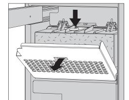
■ Loosen the filter grille and fold it downwards. Alternatively, you can also remove the grille.
