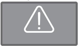
In the event of a fault, a warning symbol \( \tilde{\Lambda} \) appears on the display and the Start/Stop sensor control flashes red in rapid succession. If buzzer tones are activated, a warning tone will also sound. Warning messages must be acknowledged by tapping the warning symbol. Troubleshooting assistance can be found in \( \begin{align\*} \tilde{\Lambda} \) "Problem solving guide".
