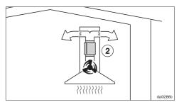
In recirculation mode the silencer needs to be positioned between the exhaust connection and the directional unit ②. Please ensure there is adequate installation space.
