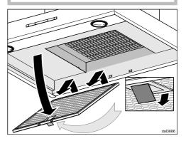
■ To take out the grease filter, release the locking clip on the filter, lower the filter approx. 45°, unhook it at the back and remove it.
