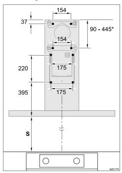
■ For pre-installation of a back wall where the holes have to be pre-drilled, please refer to the drilling distances in the drawing above (screws Ø 5 mm).
