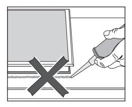
Using sealant under the cooktop could result in damage to the cooktop and the worktop if the cooktop ever needs to be removed for servicing.
