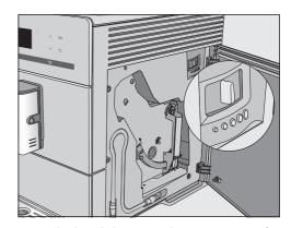
Push the slide control a maximum of one setting to the left (for finer grinding) or to the right (for coarser grinding).
