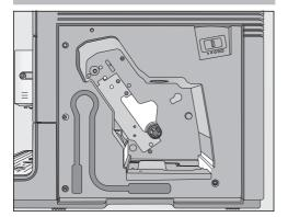
Clean the inside of the coffee machine. Make sure that the areas highlighted in the illustration are cleaned especially well.
