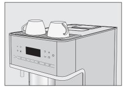
Arrange the cups or glasses on the cup heating surface on the top of the coffee machine.
