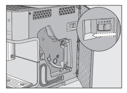
Push the slide control a maximum of one setting to the left (for finer grinding) or to the right (for coarser grinding).
