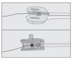
Clean also the hose connections in the rinse valve body. To do this, insert the cleaning brush into both openings and move the brush back and forth.
