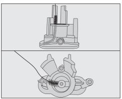
Angle the cleaning brush slightly and clean both spouts from above and below.
