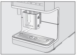
■ Push the central spout right down and remove the stainless steel cover by pulling it off towards you.
