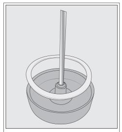
If necessary, you can remove the connecting piece and sealing ring from the milk container lid. Once you have removed the stainless steel tube, the connecting piece is easy to push out from the inside of the lid.
