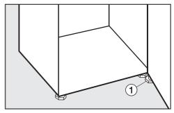
■ Ensure that you unscrew adjustable foot ① from the hinge plate until it sits on the floor. Then unscrew the foot by a further ¼ turn.
