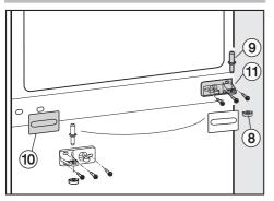
■ Remove hinge pin ⑨ from the middle of the appliance by pulling it up.
