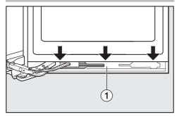
■ Loosen panel ① from the soft-close mechanism by inserting a flat-headed screwdriver into the gaps from above and, taking care, gradually lift the panel off.
