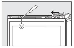
■ Use screw ③ to secure the spacer and soft-close mechanism in place.
