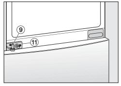
■ In the middle of the appliance, insert hinge pin ⑨ through hinge plate ⑪ and into the lower appliance door.
