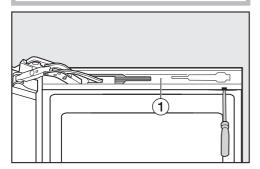
■ Loosen the panel ① from the softclose mechanism by inserting a flatheaded screwdriver into the gaps from below and, taking care, gradually lift the panel off.
