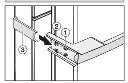
■ Loosely attach the handle to the opposite side of the door with the two front screws ①.
