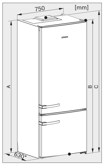
$^{\star}$  Dimensions without wall spacers. Appliance depth is increased by 35 mm with the wall spacers supplied fitted.
