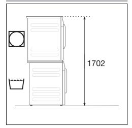
A stacking kit\* (APCL 001) is required. This must be fitted by a Miele authorised technician. Secure the washing machine using the fastening bracket supplied with the machine.
