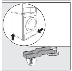
Secure 2 feet to the tumble dryer diagonally at the front and rear or only at the rear. Only the "Little Giants" models listed in the table may be installed as dryer stacks in the prescribed combinations.
