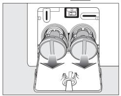
■ Remove the filters completely.
