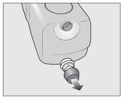
Remove the cover cap from the cartridge.
