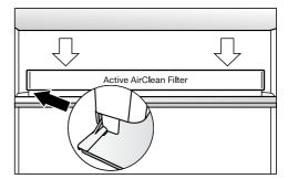
Place the holder in the middle of the protective strip at the back of the adjustable shelf so that it clicks into position.
