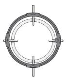
■ Place the wok ring on the pan support so that it sits securely in position and cannot move (see diagram).
