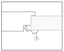
■ Secure the hob using the brackets ① supplied.
