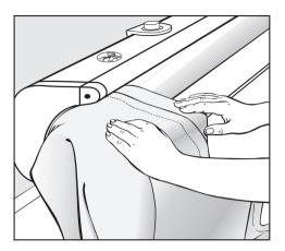
■ First do up poppers and buttons. Feed this end through the left hand side of the ironer first. Buttons should face into the roller.
