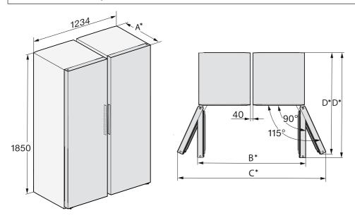
\* Dimensions without wall spacers fitted. Fitting the wall spacers supplied increases the appliance depth by 15 mm.
