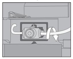
**Useful tip:** If necessary, turn the milk pipework towards the back at the connecting piece on the right-hand side.
