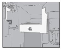
Remove the milk valve cover: press on the recessed grip to unlock the cover. On the top right-hand side of the cover, you will find a pin for swivelling the cover out.
