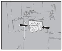
Press the retainers on the left and right-hand sides of the milk valve holder and pull the holder forward to remove it.
