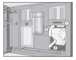
■ Pull the brew unit to the side ① first and then pull out to the front ③. Tilt the brew unit forward ② while doing so.
