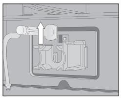
Pull the stainless steel bolt upwards and out.
