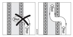
If the exhaust air is to be ducted into a flue, the ducting must be directed in the flow direction of the flue.
