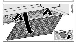
■ To take out a grease filter, release the locking clip on the filter, lower the filter approx. 45°, unhook it at the back and remove it.
