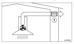
In extraction mode, the silencer not only reduces noise from the fan outside the house, but also sounds originating outside reaching the kitchen through the exhaust ducting (e.g. traffic noise). For this reason, the silencer must be positioned as close as possible to the ducting exit ①.
