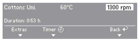
Turn the multi-function selector to highlight programme, temperature or spin speed. Pressing the multi-function selector selects the highlighted option and opens the relevant sub-menu.
