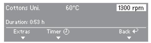
■ Using the multi-function selector you can then highlight the following options in the display: Programme, Temperature or Spin speed and confirm your selection by pressing the multi-function selector.
