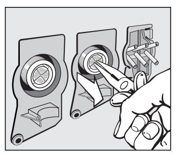
■ Use pointed nose pliers to withdraw the plastic filter by the bar (see illustration). Clean, put back and secure.
