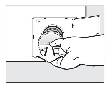
■ Remove the drain filter completely.
