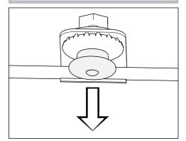
Carefully pull down the pressure cap. The browning/broiling element then lowers automatically.
