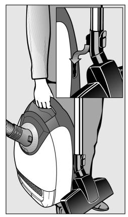
■ Slot the floorbrush downwards into one of the parking attachments on the sides of the vacuum cleaner.
