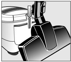
■ Slot the floorhead into the parking attachment on the vacuum cleaner.
