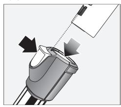
■ Insert the handle into the suction wand until it clicks into position. To do this, line up the guides on the two pieces.
