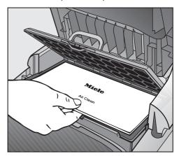
Replace it with a new AirClean exhaust filter. If you wish to fit the AirClean Plus 50, Active AirClean 50, or HEPA AirClean 50 exhaust filter, see "Replacing one type of exhaust filter with another".
