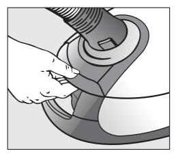
■ Press the release button on the recessed grip and raise the dust compartment lid as far as it will go.
