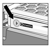
Press the TimeStrip® exhaust filter change indicator.
