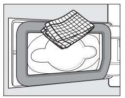
Use a damp cleaning cloth to remove any fluff. Make sure that you do not damage the rubber seal when doing this.
