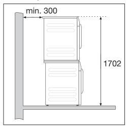
A stacking kit\* is needed. This must be fitted by a Miele authorised service technician.
