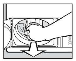
■ Use the handle to pull out the fluff filter.
