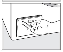
Open the access panel to the drain system.
